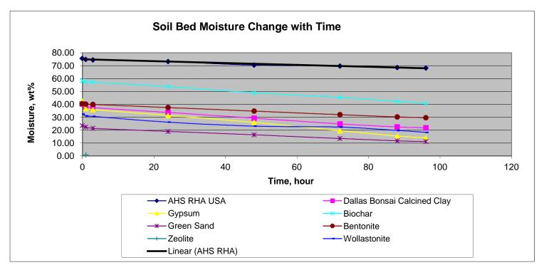
Variation of moisture of each material behaves as straight line. Slopes of each straight line indicates the rate the moisture is evaporating from the soil bed and are listed in the datasheet.
